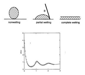
Near a repulsive wall a dense fluid of hard spheres displays pronounced oscillations on a nanoscale.
