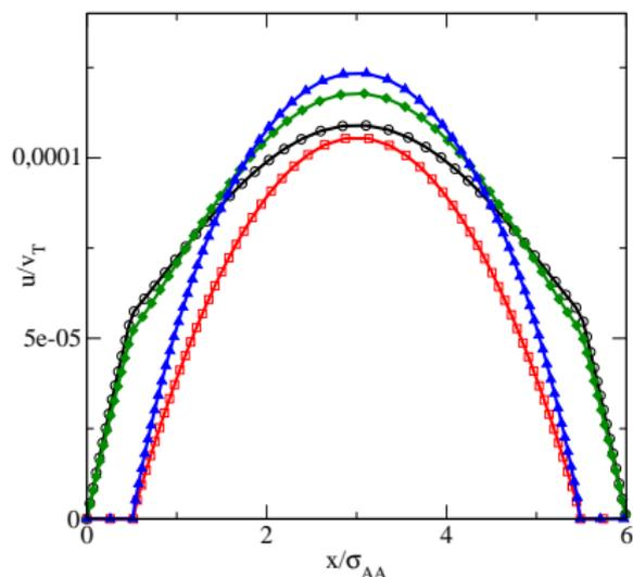
**Figure:** Velocity profiles of the two species for a channel of width  $H = 6\sigma_{AA}$  and load  $F = 0.001$ . according to the toy model.
