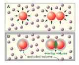
Spheres of radius R, separated a distance 2R + D, and immersed in fluid of particles with radius r,  $\mathcal{F} = -k_B T \ln V'$
