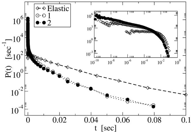
**Fig. 9.** Probability distribution functions of the collision times for the two components (system with  $r_{11} = 0.93$ ,  $r_{22} = 0.7$ ,  $r_{12} = 0.8$ ). For comparison we plotted the corresponding distributions for an elastic system. The inset shows the same curves in log-log scale
