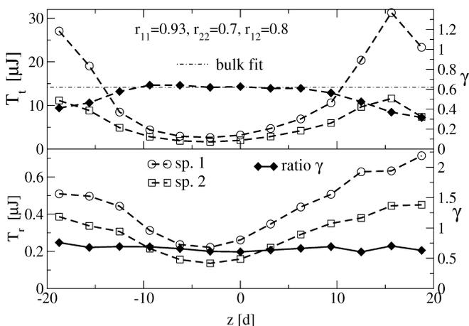
**Fig. 2.** Top panel: Translational temperature profiles for species 1 (circles) and species 2 (squares) for a mass ratio  $m_1/m_2 = 3.03$ , expressed in  $\mu\text{J}$  (left scale), and temperature ratio (diamonds)  $T_2/T_1$  (right scale). The vertical position is measured in particle diameters ( $d$ ) relative to the geometric center of the cell. Bottom panel: rotational temperature profiles for species 1 (circles) and species 2 (squares) and temperature ratio  $T_2/T_1$  (diamonds)
