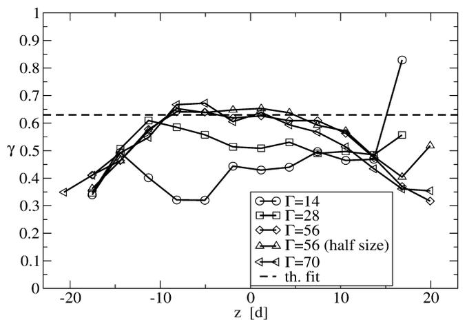
**Fig. 3.** Temperature ratio  $T_2/T_1$  profiles obtained for different values of the driving parameter  $\Gamma$  (obtained changing the vibration frequency  $\omega$ ). The particle properties are the same as those of Fig. 2 and the number of each species is  $N = 150$ , apart the upper triangles, which refer to a system containing 75 particles of each species
