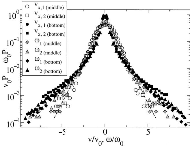
**Fig. 12.** Rescaled velocity distribution functions for the  $48 \times 64$  system measured at different heights: the system has been divided into three regions of width  $L_x$  and height  $L_y/3$  and the distributions of the translational and rotational velocities of the grains in the bottom and middle regions have been calculated
