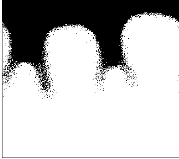
Figure 1: The combustion field at t = 16000 MCS. The initial oxygen concentration is A_0 = 0.90 , the frequencies of attempt for the heat and the oxygen fields are f_H = 0.2 and f_O = 1 respectively, the heat threshold is S_H = 0.50 .
