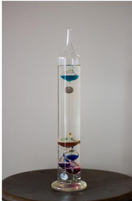
**Fig. 1.** An example of Galileo's thermometer: the room temperature has an uncertainty of  $1^\circ\text{C}$ .
