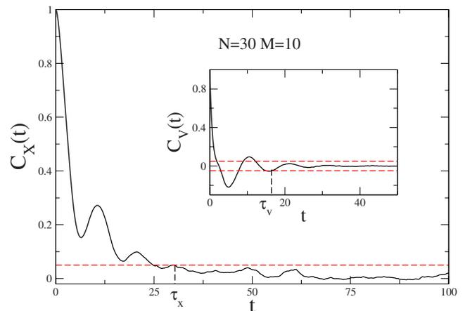
Fig. 4. (Color online) The autocorrelation function of the position  $X$  and velocity  $V$  of the piston for  $N=30$ ,  $M=10$ ,  $F=10$ ,  $T=1$ , and  $m=1$ . The estimates of the correlation times  $\tau_X$  and  $\tau_V$  are shown. Although the two correlation functions  $C_X(t)$  and  $C_V(t)$  are different, the corresponding characteristic times are of the same order.
