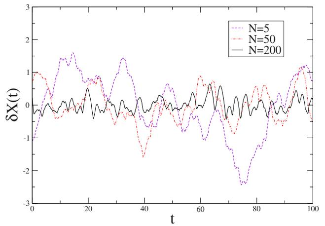
Fig. 2. (Color online) Time series of the displacement of the piston from its mean value for different values of  $N$ . The other parameters are  $M=10$ ,  $F=10$ ,  $T=1$ , and  $m=1$ . One can see that, although the qualitative behavior does not change with  $N$ , the amplitude of fluctuations decreases with  $N$ .
